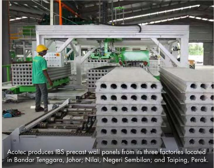
Acotec produces IBS precast wall panels from its three factories located in Bandar Tenggara, Johor; Nilai, Negeri Sembilan; and Taiping, Perak.
